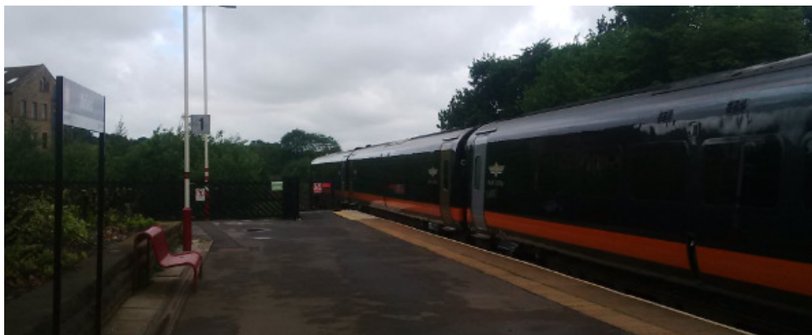
Figure 22: Mirfield – this Grand Central train has stopped with the last (wheelchair-accessible) carriage off the platform
