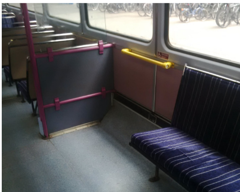
Figure 10: Class 142 interior showing non-compliant wheelchair space
