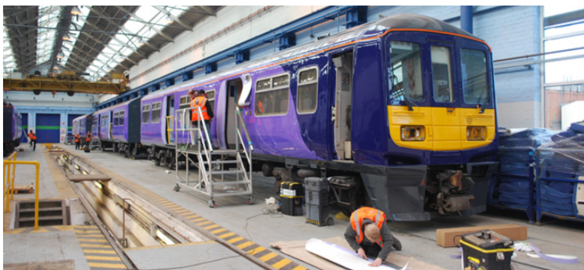
Figure 37: This ex-Thameslink Class 319 train is being refurbished for use on newly-electrified routes in the North of England (source Northern website)
